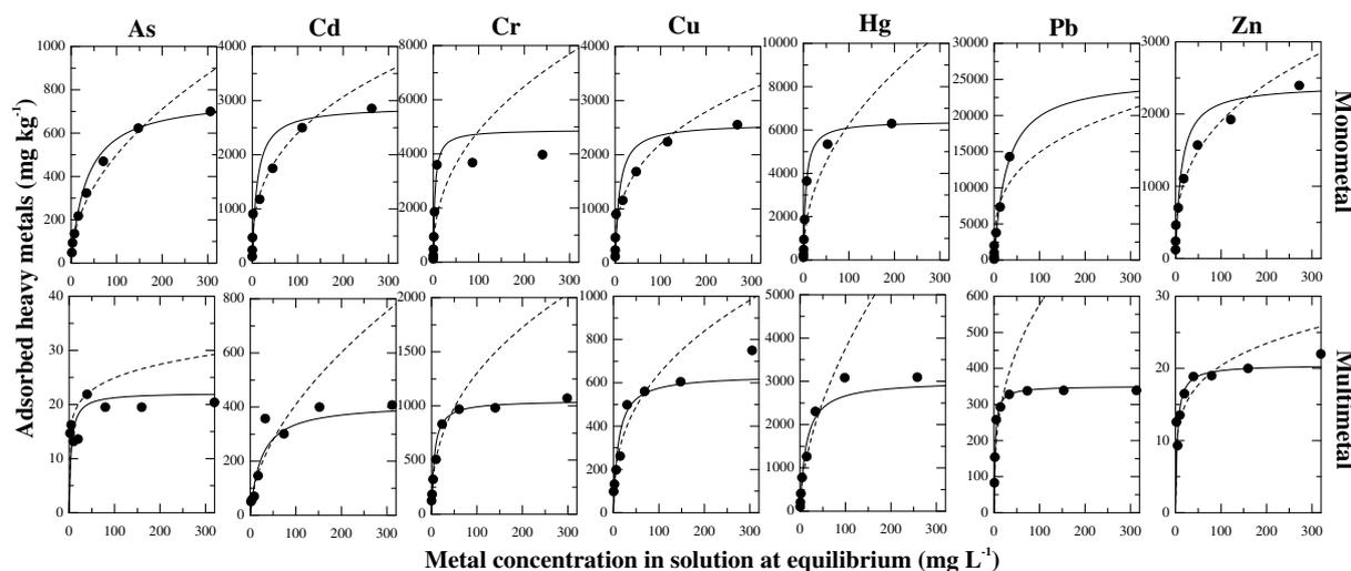
**Fig. 1.** Experimental and calculated values from the Freundlich and Langmuir adsorption isotherms for the monometal and multimetal conditions. ●: Experimental data; —: Langmuir equation (Eq. (3)); - - -: Freundlich equation (Eq. (1)).
