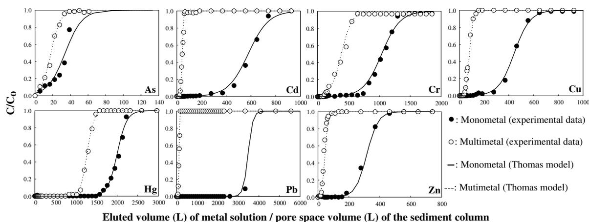
Fig. 2. The experimental and predicted breakthrough curves using the Thomas model in the monometal and multimetal columns.
