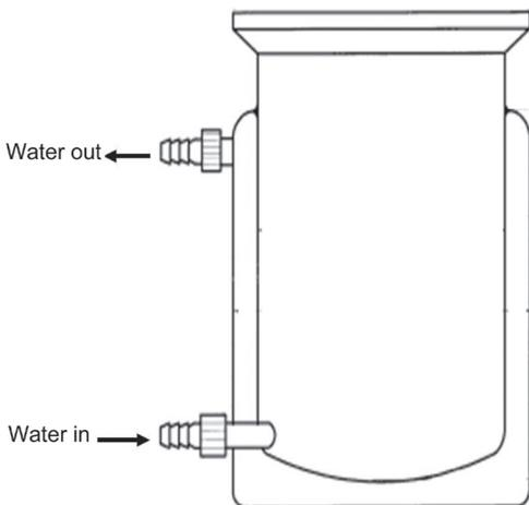
Fig. 7-2. Heatproof flat-bottomed glass reaction vessel with thermal jacket.
