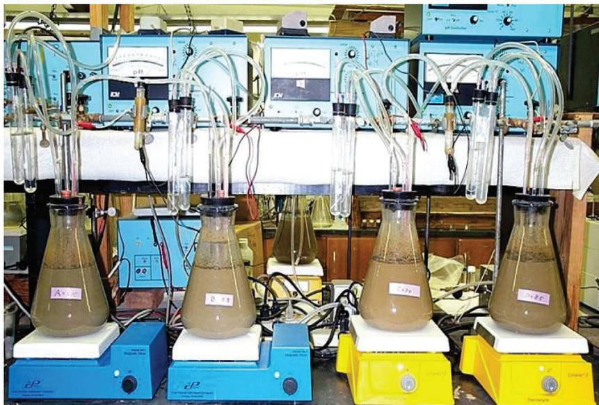
Fig. 7-1. Basic components of a redox potential–pH controller (top) and its photograph (bottom) (modified from Yu and Rinklebe, 2011).
